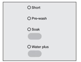
Press the appropriate additional option button. Press the top button repeatedly until the indicator light for the additional option you want comes on.
